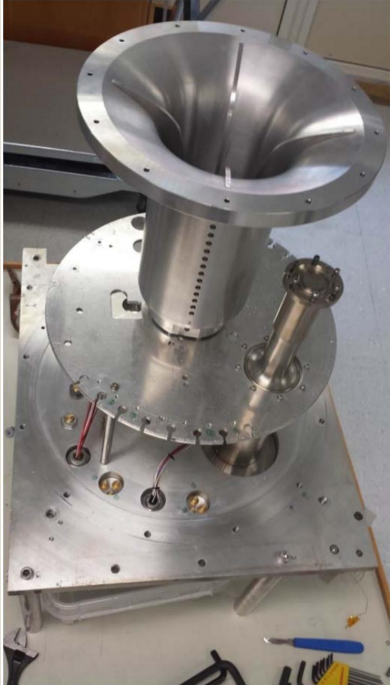
Quad-ridge feed horn as tested
